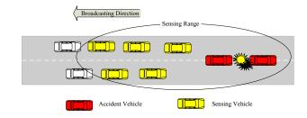
Fig. 1. Emergency Event Sensing in VANETs
